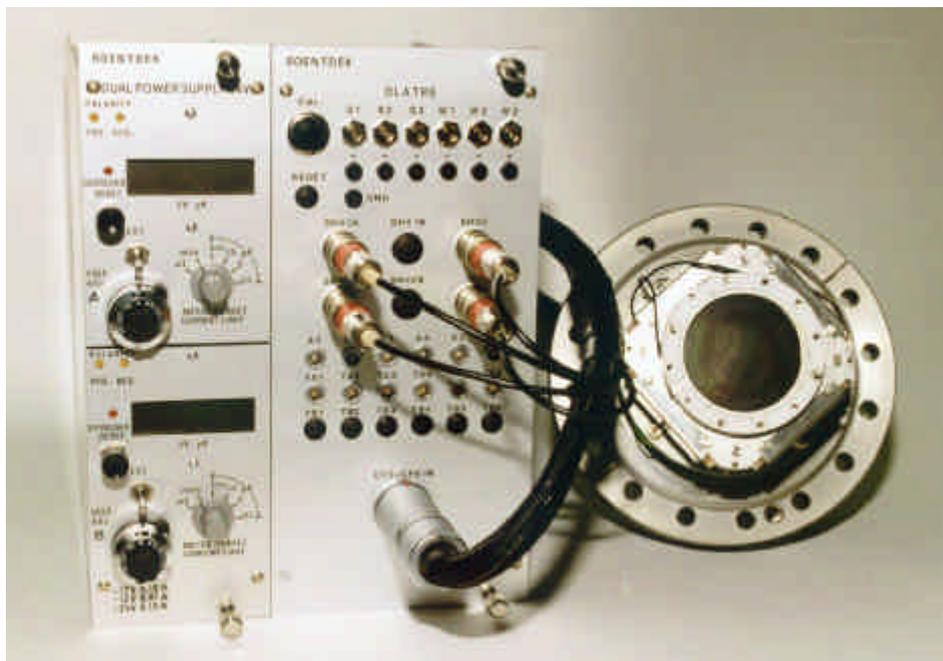
*Figure 4: Components of the delay-line detector system. Right to left: MCP-detector with delay-line anode (active diameter 45 mm) mounted on CF100-flange with feed-through, front-end electronics box and specially developed power supply unit with two independent channels, +/- 4 kV, trip protected.*
