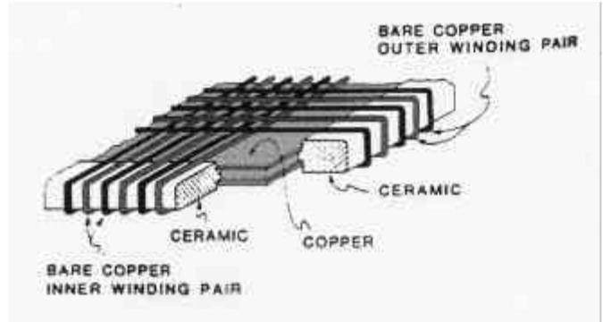
Figure 2: Corner detail of a helical wire delay-line anode<sup>12</sup>
