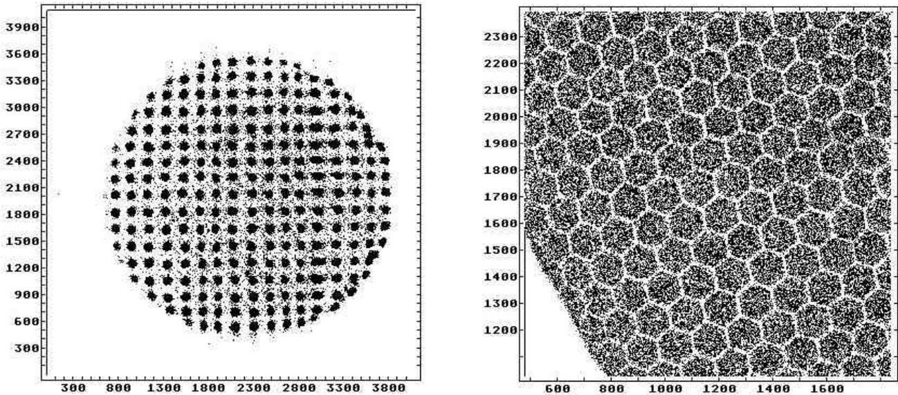
Figure 5: Imaging performance of the delay-line detector/front-end box investigated by irradiating a MCP-stack with an  $\alpha$ -source. A TDC with 50 picosec resolution has been used here. The MCP have a pore size of 25  $\mu\text{m}$  (center-to-center 32  $\mu\text{m}$ ), an L/D of 40, “detection quality”.
