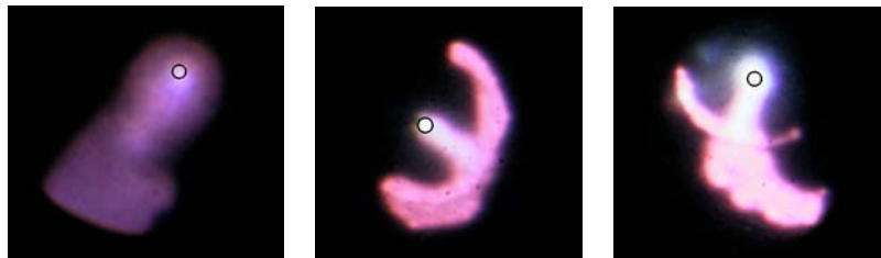
Figure 3.13: Contraction of the homogeneous glow discharge, incipient (a) and filamentary discharge (b and c).
