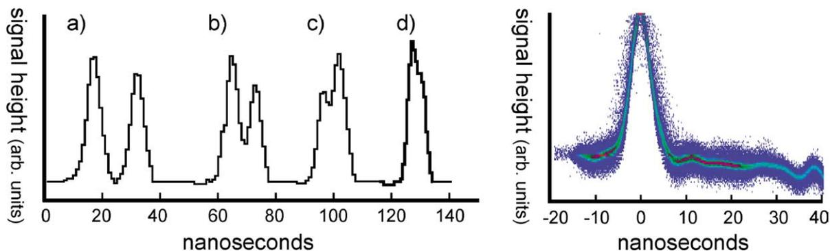
Fig. 7. Left part: Double peaks with different spacing. Even case (d) can be resolved as two peaks using pulse fitting methods. Conventional TDC-systems combined with constant-fraction discriminators do not reach this performance. Right part: Several hundred normalized pulses are plotted in the same histogram. The shape of the signal is apparently independent from the pulse height which is a prerequisite for the fit algorithms.
