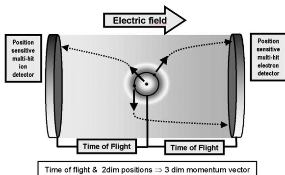
Fig. 1. Scheme of the COLTRIMS imaging system [2].
