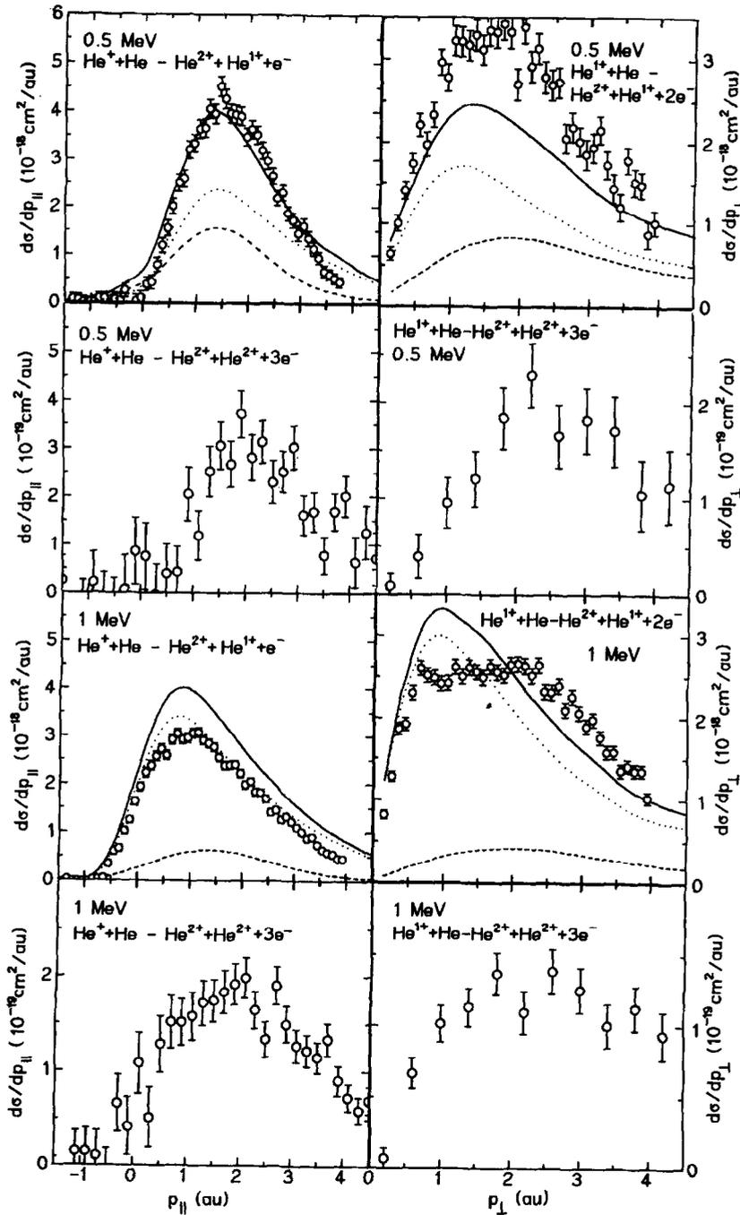
Fig. 2. Single differential cross sections for reactions (1) and (2). Left column: longitudinal momentum distribution. Lines: two center nCTMC calculation; dotted line: sum of (ee) and (Ne) contribution; dashed line: double ionisation plus capture (see text); full line: sum over both processes. Right column: perpendicular momentum distribution.
