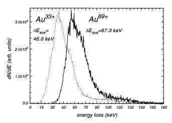
FIG. 1. Energy-loss distributions of Au<sup>33+</sup> and Au<sup>69+</sup> after transmission through a thin carbon foil ( $\Delta x \approx 10.4$  nm). The initial energy was 454.4 (±3) keV.
