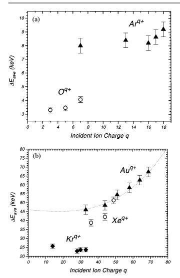
FIG. 2. Average energy loss of (a)  $O^{3,5,7+}$  and  $Ar^{7,13,16,17,18+}$ ; (b)  $Kr^{14,28,30,33+}$ ,  $Xe^{36,44,49+}$ , and  $Au^{33,44,51,58,64,69+}$  in a thin carbon foil. The dotted line is a fit to the  $Au^{q+}$  data using Eq. (1) with n = 1, m = 2 ( $\alpha = 0.0165$ ,  $\beta = 8 \times 10^{-5}$ ).
