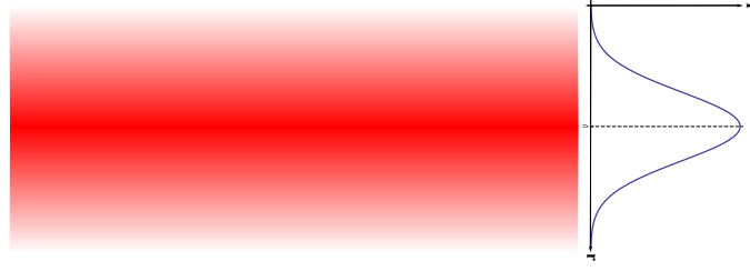
Figure 2.4: Gaussian intensity distribution of the beam (own figure)
