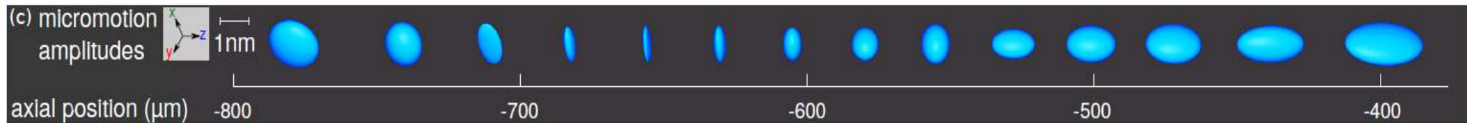
Atomically resolved micromotion of individual ions
